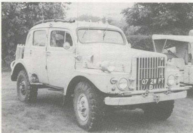
A preserved Volvo Sugga four-wheel-drive staff car attending a Tank Museum rally in 1988. Known officially as the P2104/TP21, these cars served the Swedish Army from 1953 as command staff and radio vehicles. They were powered by a straight six-cylinder side-valve engine driving through a four-speed two-ratio gearbox to the rear axle or both axles as required.
